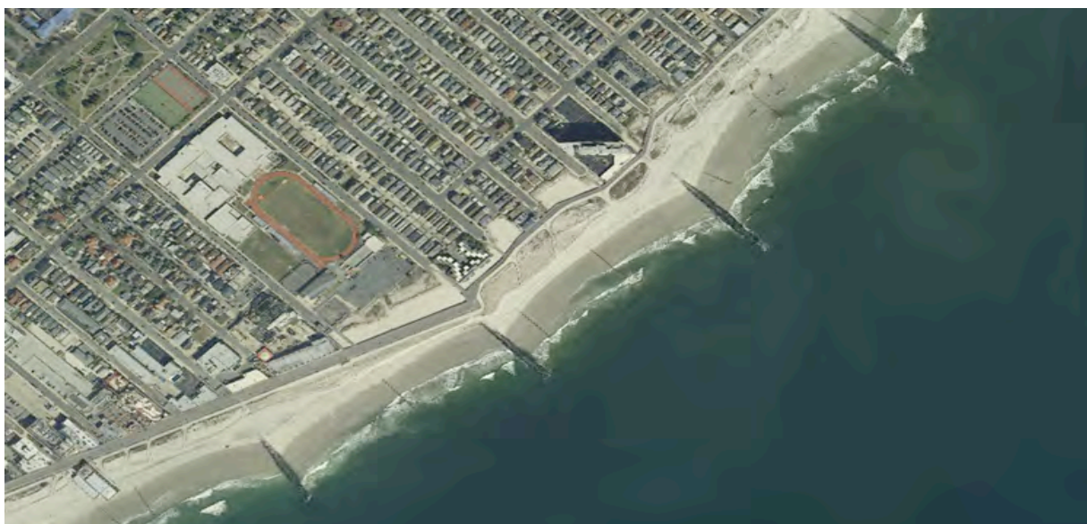
FIGURE 7: Orthoimagery of the groins along Ocean City, NJ (Cornell et al., n.d.).
