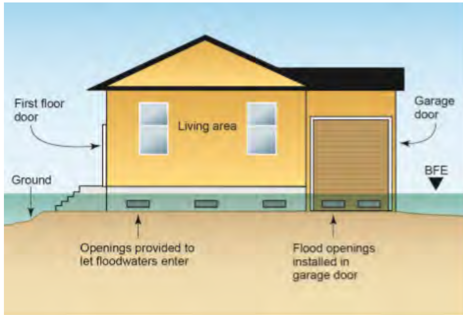
FIGURE 11: Placement of flood openings (FEMA, 2015).
