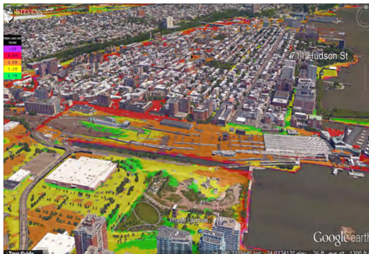
FIGURE 11: An example of an Animated Street Level Model Output of the proposed SC Model System to be time and space sequenced and then communicated with GIS overlays to the public using a smartphone app.
