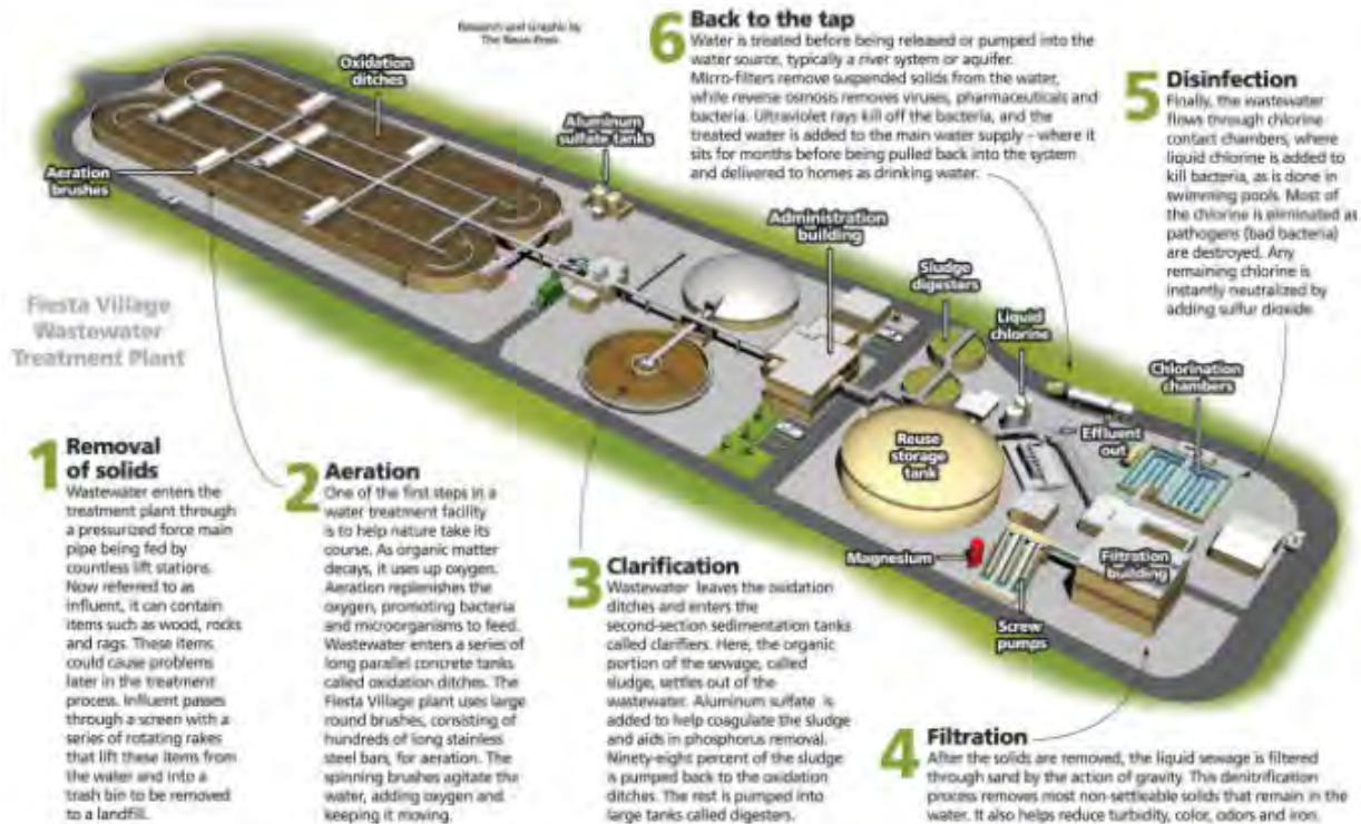
FIGURE 19: An illustration of a wastewater treatment plant in Florida (Wastewater Recycling, 2018).
